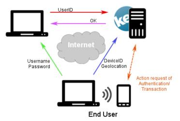
The **Keypasco Service** is based on different components, the software clients: Vakten for Desktop, Smartphone, Tablet and Browser, and the back-end server Borgen. All versions of Vakten provide a two-channel structure for secure authentication and secure notifications.
